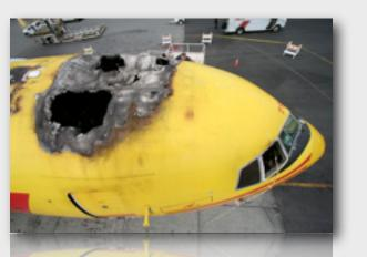
damaged the airplane. The NTSB noted that Boeing had identified safety issues involving the conductive hoses and issued a Service Bulletin calling for their replacement.
